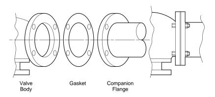
Figure-5 Installation of Flanged End Valves.
