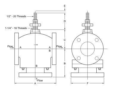
Figure-10 Typical of VB-9313-0-5-P, 2-1/2" to 6" Valve Bodies.
