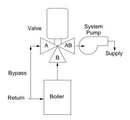
Figure-7 Typical Boiler Hot Water Reset.
