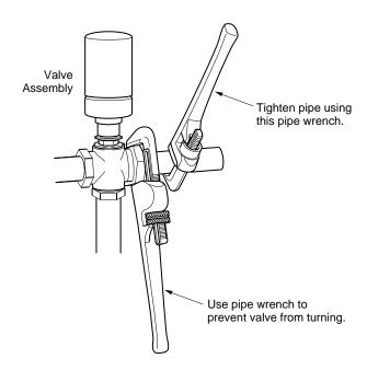
Figure-4 Installation of Screwed End Valves.
