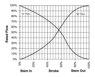
Figure-1 Typical Flow Characteristics.
