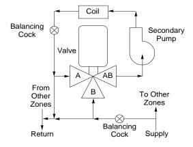
Figure-8 Typical Primary-Secondary Piping.
