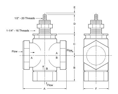
Figure-9 Typical of VB-9313-0-4-P, 2-1/2" and 3" Valve Bodies.
